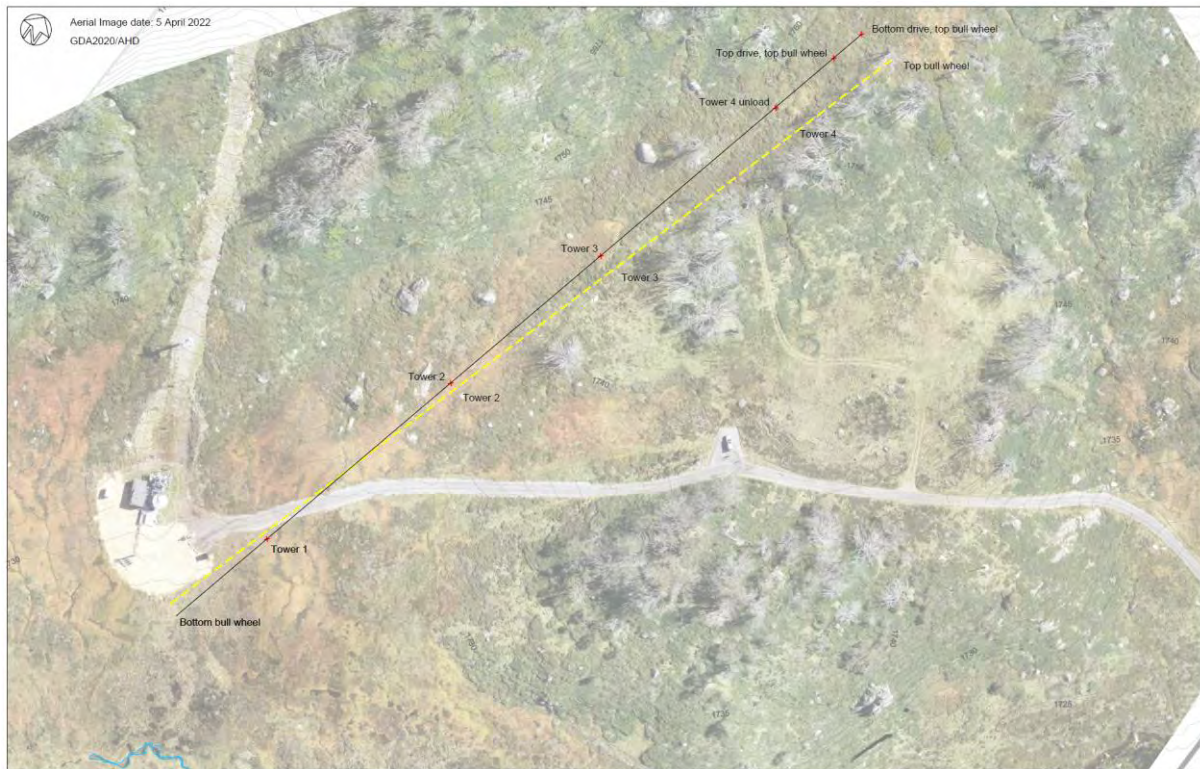
Figure 12: Original preferred lift alignment (black) and proposed modified lift alignment (yellow)
